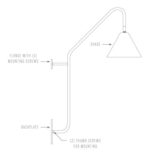
\*THIS FIXTURE IS WIRED THROUGH THE BOTTOM BACKPLATE
